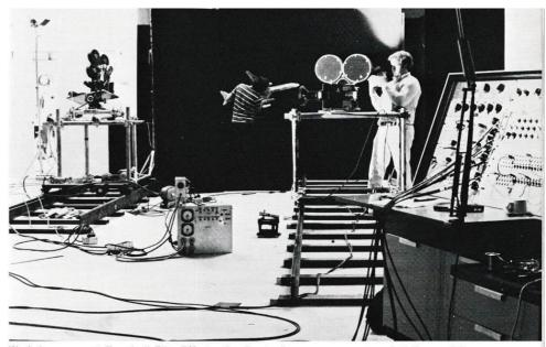
Work in process at Trumbull Film Effects, showing tracks, camera mounts and dollies used for slit-scan and other effects. Artist is painting airplane model matte white so that automatically matched movement can be shot to produce high-contrast, bi-pack matte.
